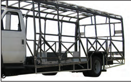
1½" x 1½" Steelguard® construction provides superior durability.
