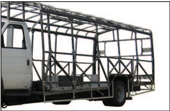
1 1/2" x 1 1/2" Steelguard® construction provides superior durability.
