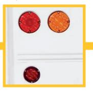
LED clearance lights, direction lights and stop lights are standard equipment offering enhanced safety, while reducing operating and maintenance costs.
