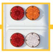
LED clearance lights, direction lights, stop lights and back-up lights are standard equipment offering enhanced safety, while reducing operating and maintenance costs.
