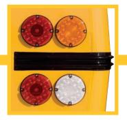
LED clearance lights, direction lights, stop lights and back-up lights are standard equipment offering enhanced safety, while reducing operating and maintenance costs.
